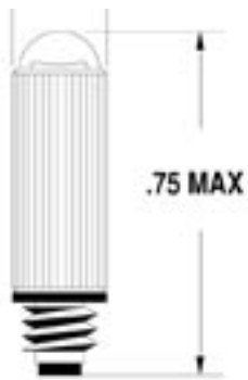
8-35 UNC 2A Thread 2.5V .30A 15 Hour Life Nickel Plated Vacuum TL-1 1/4 Lamp
